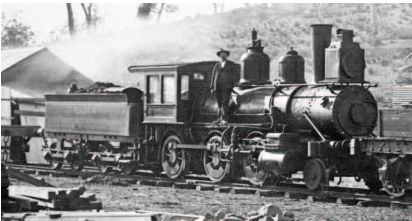
Baldwin 5ft 3in gauge 2-6-0 locomotive MAJOR (B/No. 10067 of 1889) at McIvor Siding, c. 1906. MAJOR and its identical mate McIVOR were light and flexible and perfectly matched for the task. Photo: courtesy Miss Mavis Prince
