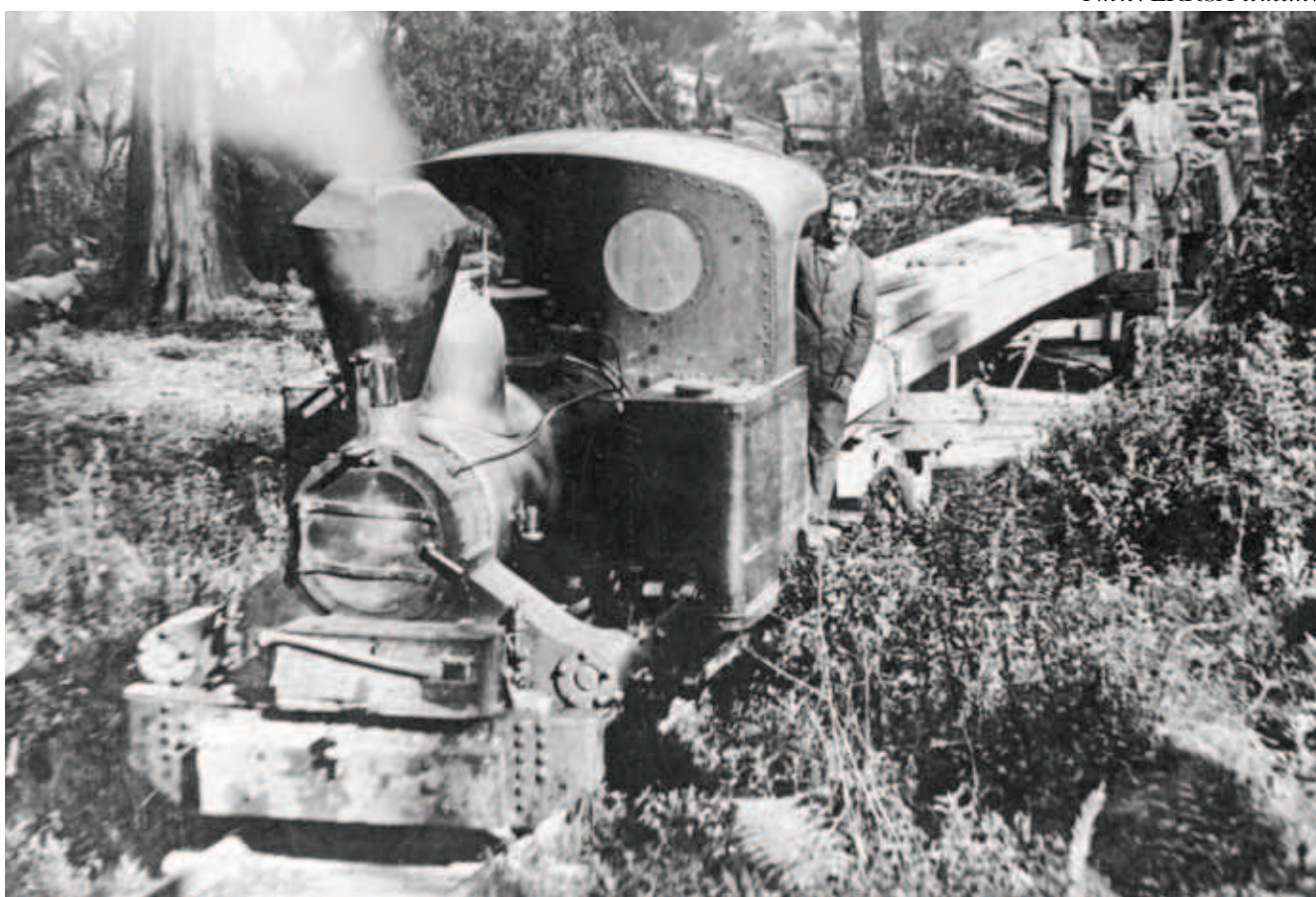
Fowler 3ft 6in gauge 2-4-0T patent jack-shaft drive locomotive PARROT (B/N. 4150 of 1881) at work on Sanderson's tramway, hauling sawn timber from his Noonday Creek mill, c. 1899. It was supplied for sugar plantation use and was found to be under-powered for timber tramway work.
