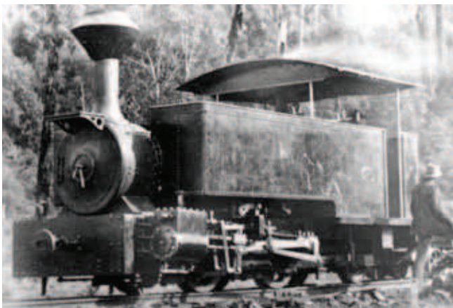
Fowler 3ft gauge 0-4-2T (B/No. 13576 of 1913) of the Warburton Timber and Tramway Co. between Warburton and Big Pats Creek. It was a 3ft gauge version of a standard 2ft gauge Fowler design used on Queensland sugar tramways, even having a tropical cab, which was not well suited to the Warburton climate.
