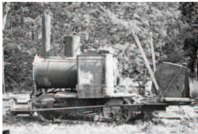
Ex Bendigo Tramways Phoenix steam tram motor converted from standard to 3ft 6in gauge out of use on WW Gunn's crossover tramway c. 1936. Though not built for timber tramway use, it performed well.
