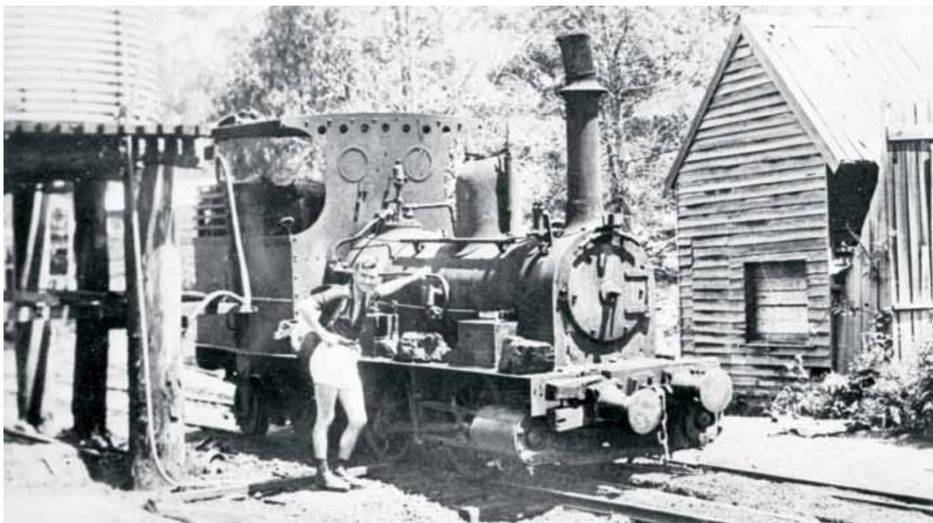
Ex-South Australian Railways 3ft 6in gauge 0-4-4WT (James Martin B/No. 67 or 69 of 1893) at Goodwood, c. 1934. Photo: LRRSA collection □ Sharp Stewart 3ft 6in gauge 0-6-0ST (B/No. 2030 of 1870) on the Elphinstone tramway c.1925. It had been rebuilt from a 4ft 6in gauge 0-4-0ST originally built for the Mersey & Deloraine Tramway in Tasmania. Photo: LRRSA collection □ Goodwood tramway 3ft 6in gauge 2-6-0 at Noojee in 1936. The Beyer Peacock 2-6-0 with leading Bissell truck was a very successful type, which was used in every Australian state and the Northern Territory. This (B/No. 2245 of 1882) was the only one to work in Victoria. It was an extreme example of the rough life experienced by steam locomotives on timber tramways. At some time it had lost its tender and ended its working life in a bridge collapse in 1936. But it had already experienced at least one bridge collapse on the Goodwood tramway, which was possibly when it lost its tender. Photo: John Buckland
