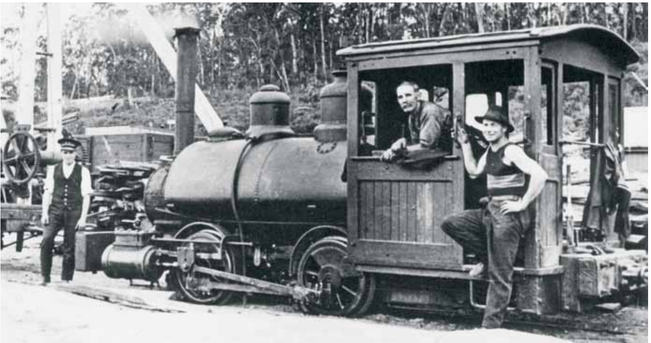
Baldwin 3ft 6in gauge 0-4-0ST (B/No.9086 of 1888 or 12007 of 1891) working on the Loch Valley Timber Company's tramway at Noojee station, c.1923. The working life of both locomotives ended in 1926 when they were badly damaged in a bushfire. Photo: LRRSA collection
