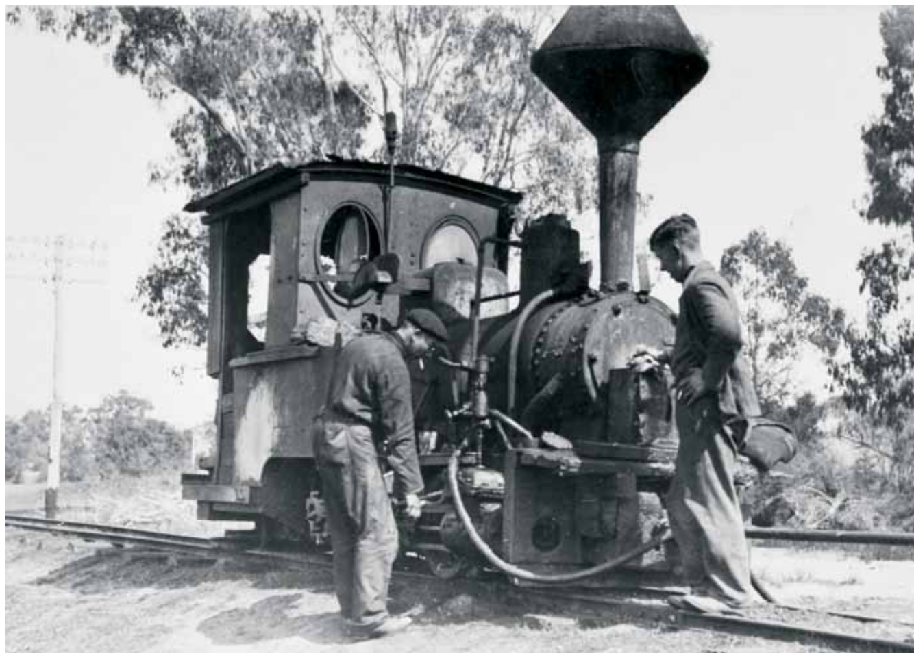
Krauss 2ft gauge 0-4-0WT (B/No. 2459 of 1891) takes water on the Rubicon – Alexandra tramway in 1934. The driver, Bob Rees attends to the engine, while brakeman Hayden looks on.
