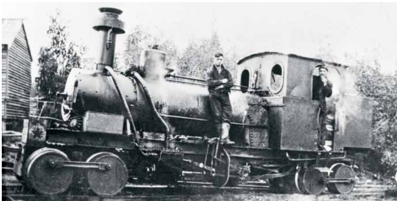
3ft gauge 0-4-4-0 geared locomotive built by Day's Engineering seen on Jack Ezard's Starvation Creek tramway, east of Warburton. The driver is N Hooper, and the fireman is T Hill. Photo: LRRSA collection
