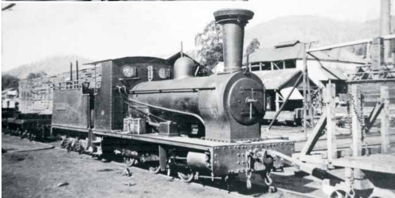
Baldwin 3ft gauge 2-4-0 LITTLE YARRA (B/No. 37718 of 1912) at Powelltown, c. 1937. The back of the tender has been dented as a result of a shunting accident, and the rails on the top of the tender have become very battered. Photo: JCM Rolland □ Kerr Stuart 3ft gauge 0-4-0T locomotive Coffee Pot (B/No. 643 of 1898) at Powelltown c.1937. The loco was painted green and traces of lining on the tank sides appear to be visible. Photo: JL Buckland □ Bagnall 3ft gauge 0-6-0 POWELLITE (B/No. 1965 of 1913) at Powelltown c.1937. The oversized funnel was fitted in the late 1930s by the Victorian Railways when the loco was overhauled at Newport Workshops, and in this view the pancake shaped object on top appears to be a Cheney spark nullifier. Photo: JCM Rolland
